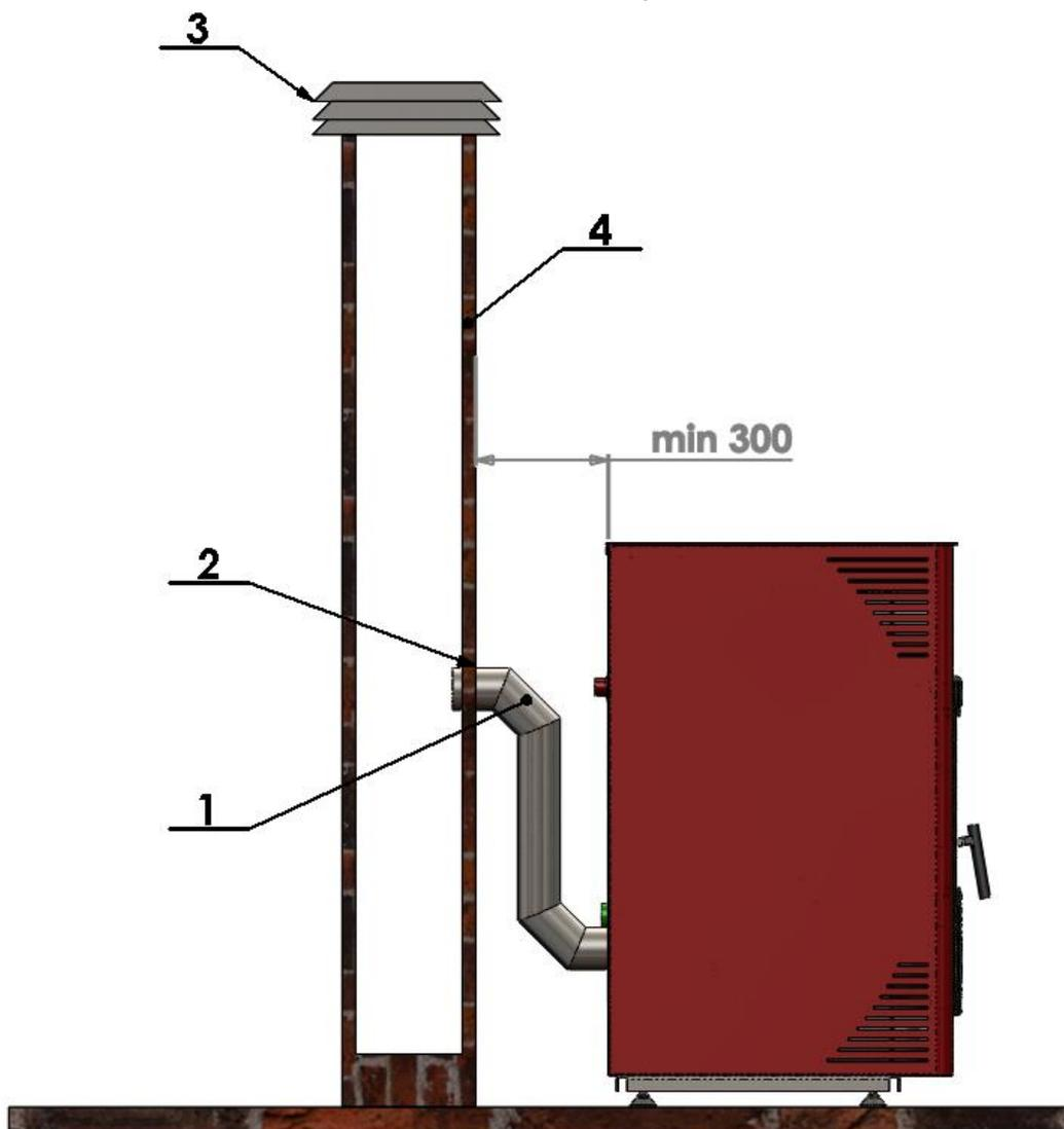
1) Flue pipe 2) Gasket 3) Fireproof protection cap 4) Chimney diameter not greater than
