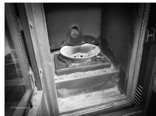
The heating chamber must be free of ashes when finished.
