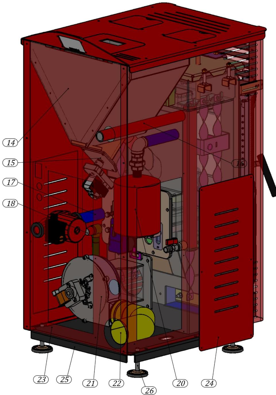
14. Pellet magazine 15. Pellet feeding auger with motor 16. Flow line 17. Circulation pump 18. Safety valve
