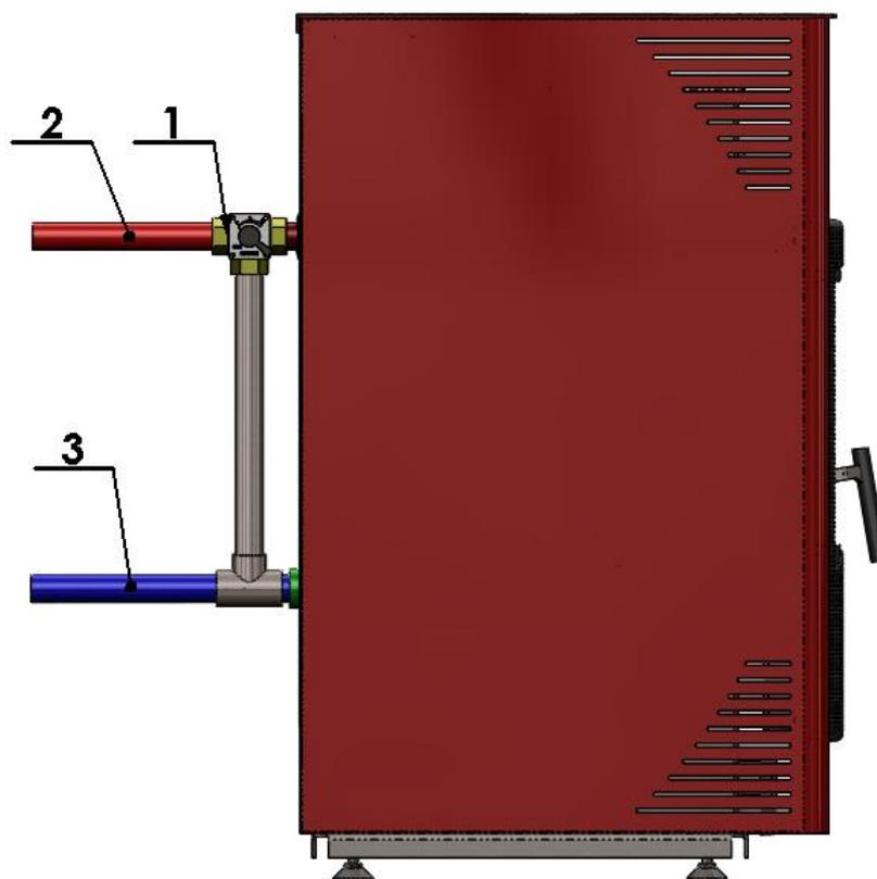
1. 3-way mixing valve 2. Circulation pump 3. Thermostate
